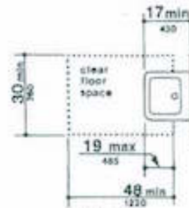
Fig. 32 Clear Floor Space at Lavatories
